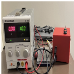
Figure 3.1: (a) – Waveflap driven by servo motor (red); (b) – Power supply and control box, green button generates waves, switch allows manual waveflap adjustments; (c) – Buoy, V-channel and induction coils (red) setup.
