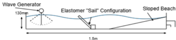
Figure 5.1 - Schematic of the elastomer energy harvesting experimental setup including sloped beach absorber position.
